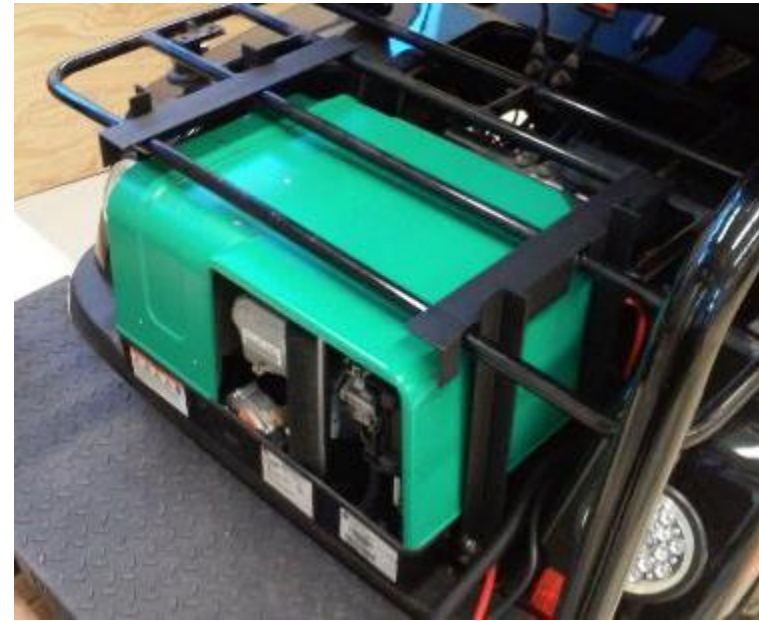
Figure 11. Photograph of generator mounted to rear of cart.
