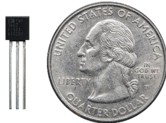
Figure 15. TMP Sensor. Quarter for scale [6]
